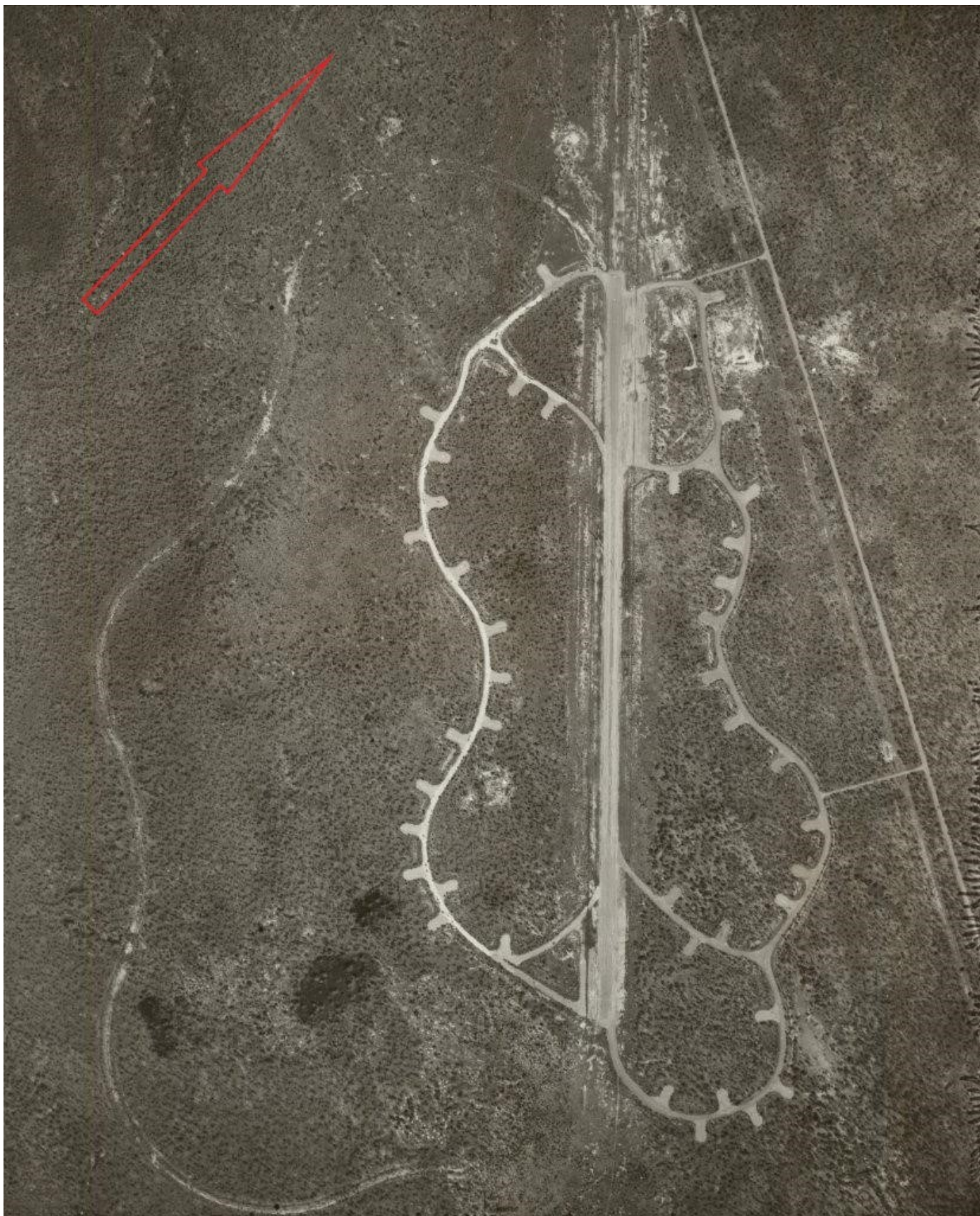
"Tindall A/F" taken by 1SQN on 25 th February, 1960, from 14,000 feet. The movement area at this time was apparently still in excellent condition although the graded, 2500-foot, runway extension had become over-grown. Even the path of the future dispersal taxiway, at left, was still clearly visible. Red arrow at top left indicates the direction of north. [ National Library of Australia, Australian Aerial Photographs, D 53 9 106, nla.BibID 5714725 ].
